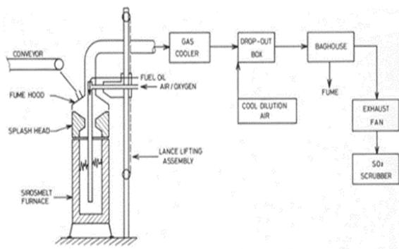
Gambar 2.2 The 50 kg SiroSmelt Pilot Plant [2]
