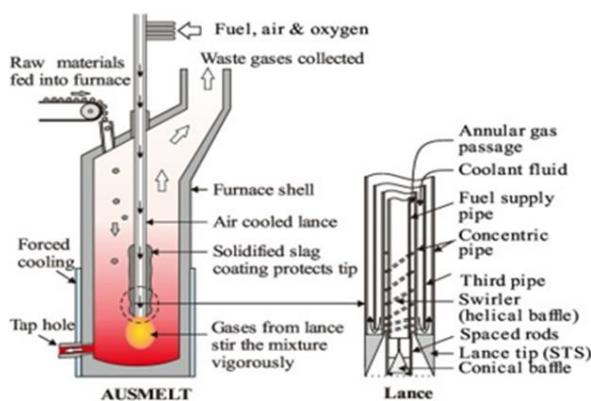
Gambar 2.2 Proses Peleburan Top Submerged Lance Ausmelt [3]
