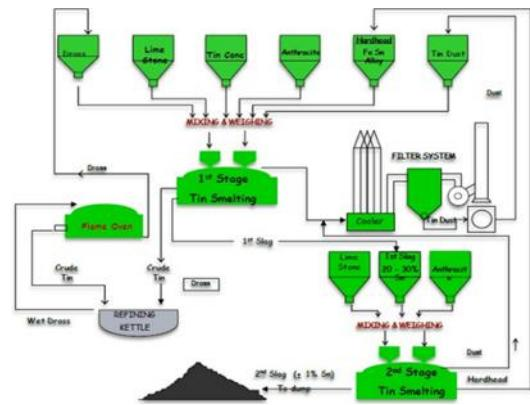
Gambar 2.1 Proses Peleburan Eksisting PT Timah Tbk[1]
