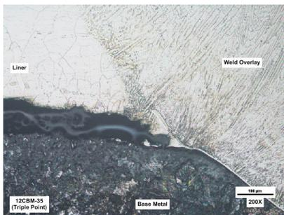
Gambar 4. 8 - Foto mikro 200x pembesaran – Triple Point / transition Weld
