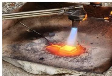
Gambar 4. 4 Proses hardening baja SKD 11
