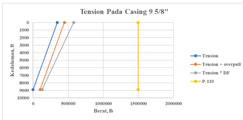
Gambar 7. Tension Design Intermediate Casing 9-5/8"
