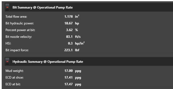
Gambar 2. 27 Hydraulics Summary (Bit Hydraulics)
