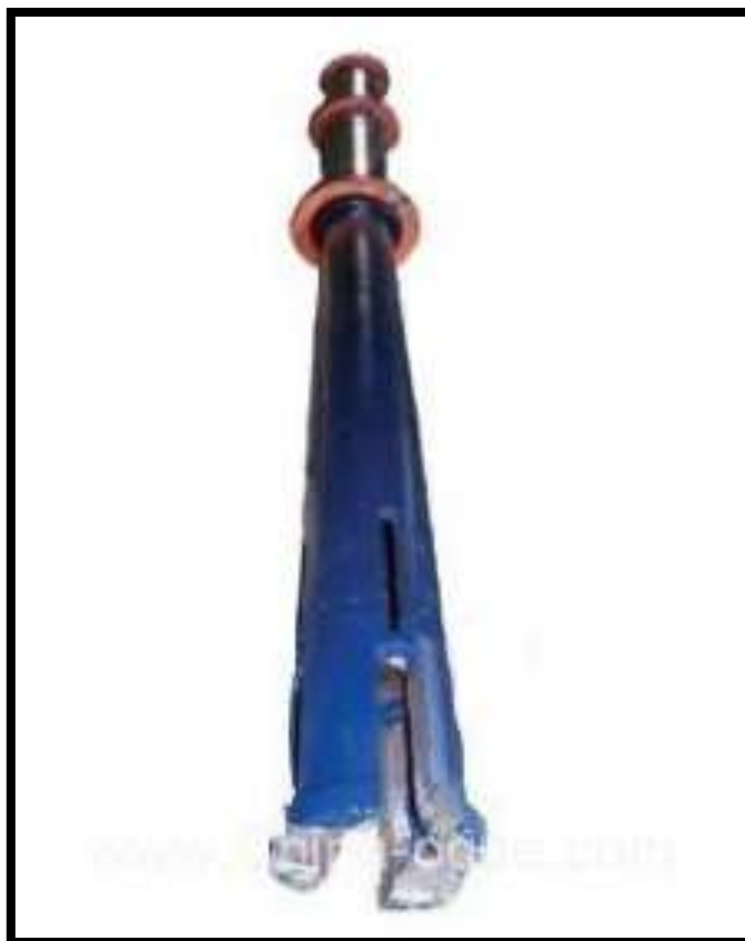
Gambar 4.4 Sand Bailer / Sand Pump.
