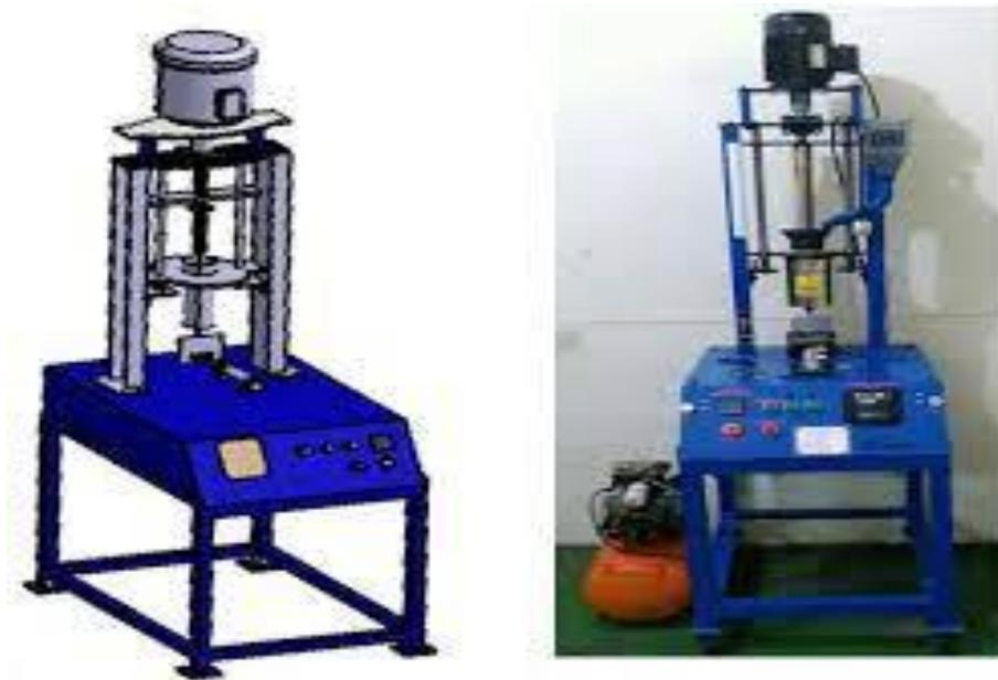
Gambar 2.2 mesin injection molding vertical
