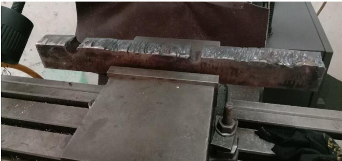
Gambar 4.9 Proses Machining Tuas
