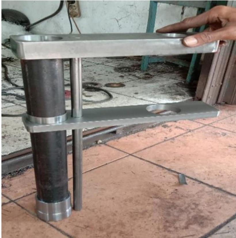
Gambar 4.15 Perakitan mesin *vertical plastic injection molding*
