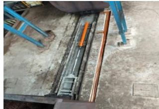
Gambar 2.2 Hydraulic indexer system
