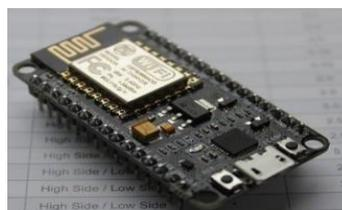
Gambar 5. NodeMCU Esp8266 [16]
