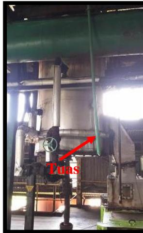
Gambar 1.2 Posisi Tuas Penggerak *Sliding Door Digester* SBYM.
