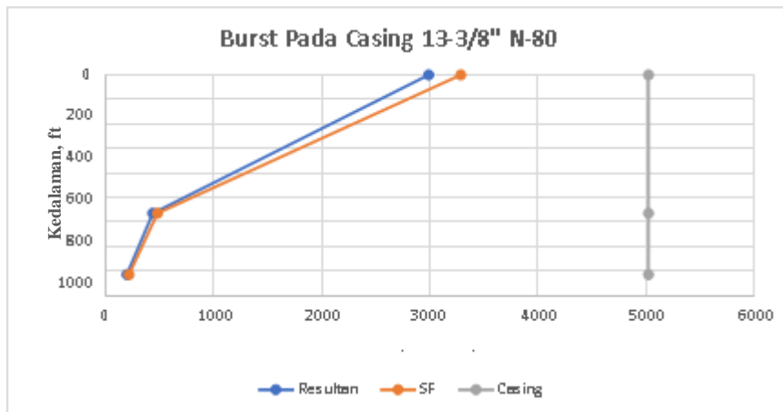
Gambar 2. Burst Design Surface Casing 13-3/8"
