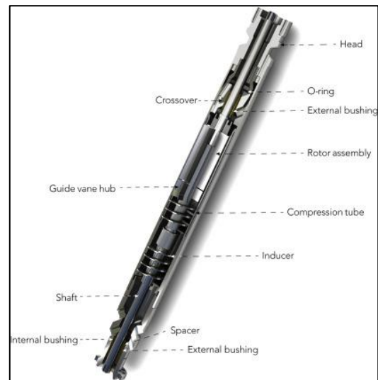
Gambar 2. 9 Jenis Rotary Gas Separator
