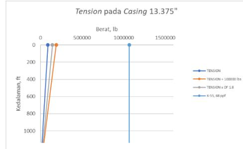
Gambar 4. Tension Casing 13.375"
