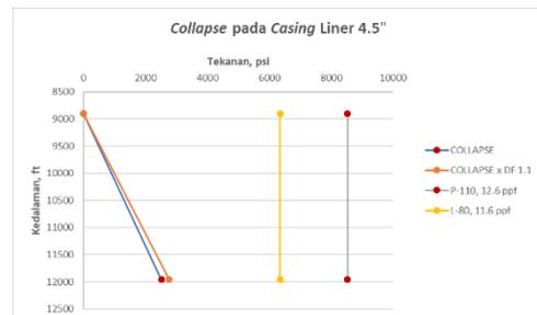
Gambar 12. Collapse Casing 4.5”
