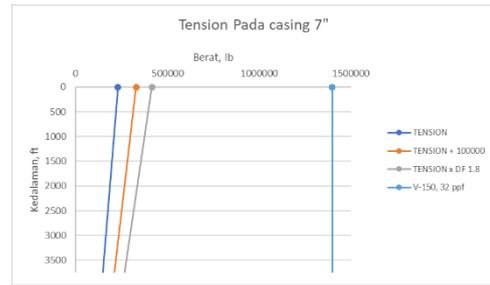
Gambar 10. Tension Casing 7”
