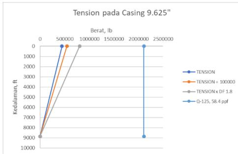
Gambar 7. Tension Casing 9.625”
