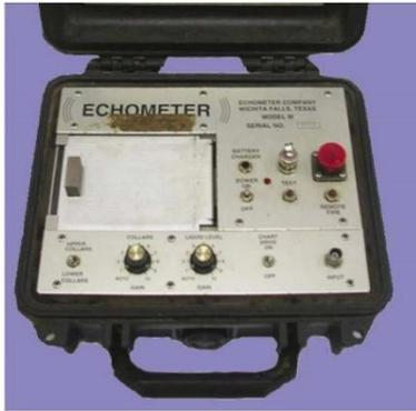
Gambar 3 Instrumen *Chart Recorder*
