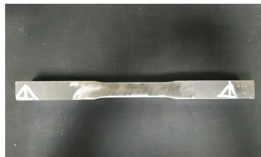
Gambar 5: Spesimen *Tension Tests*
