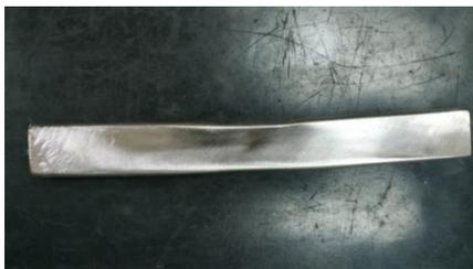
Gambar 7: Spesimen Bend Tests
