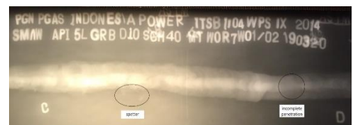
Gambar 3.4 Film radiografi hasil lasan repair welding 7x
