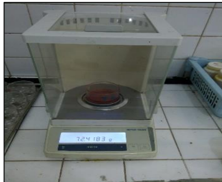
Gambar 3.4 Proses Penimbangan Sampel Basah
