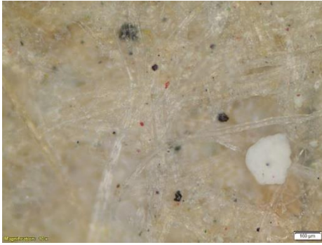
Gambar 10. 15% Deinking Sludge + 7 Kg/T Cationic Starch
