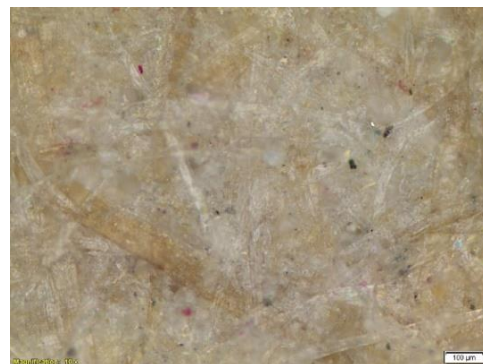
Gambar 9. 10% Deinking Sludge + 5 Kg/T Cationic Starch
